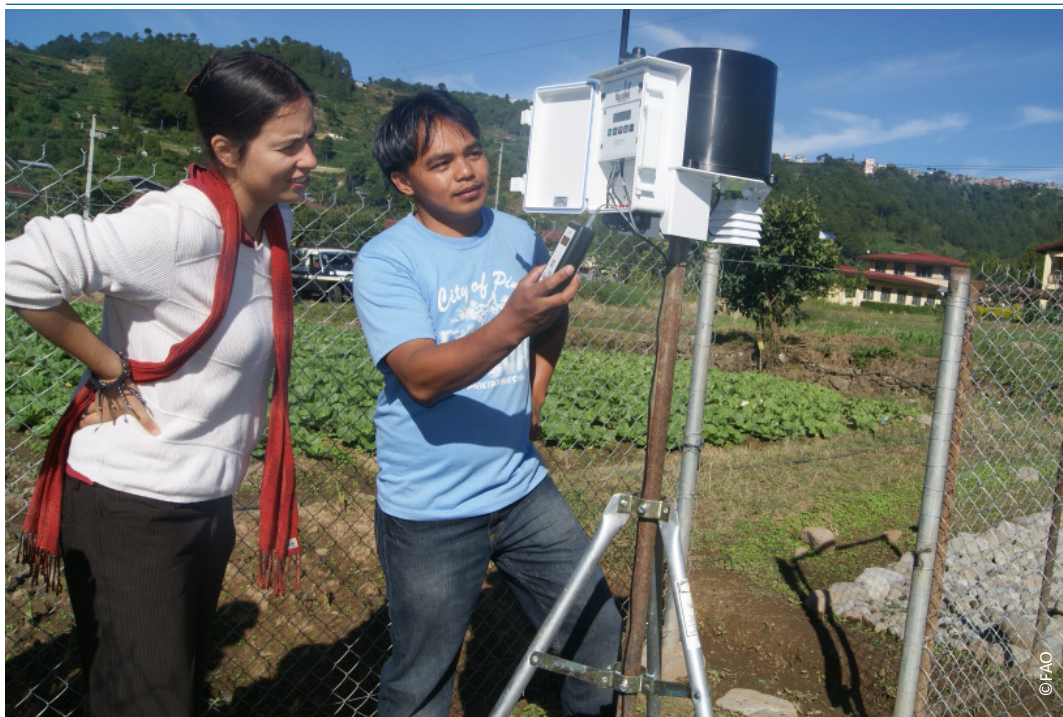
Climatic data being downloaded from an automatic weather station (AWS) installed at Benguet State University Buguias Campus under the MDGF-1656 project on “Strengthening the Philippines Institutional Capacity to adapt to Climate Change”
